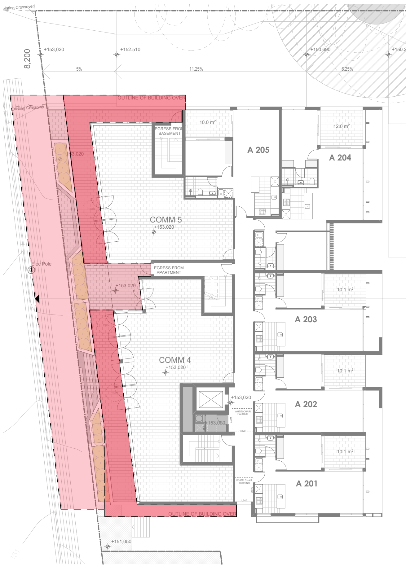
DCP Requirement - 3m Continuous Awning Beecroft Rd
